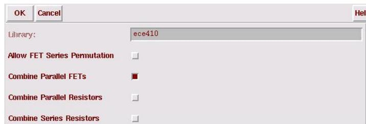
You should confirm this setting before performing LVS on most logic gates that are more complex than the INV cell, including NAND and NOR gates.
