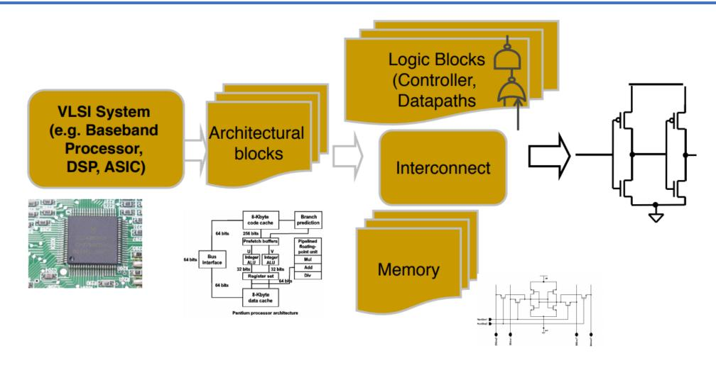
System -> Architecture -> Logic -> Transistor
